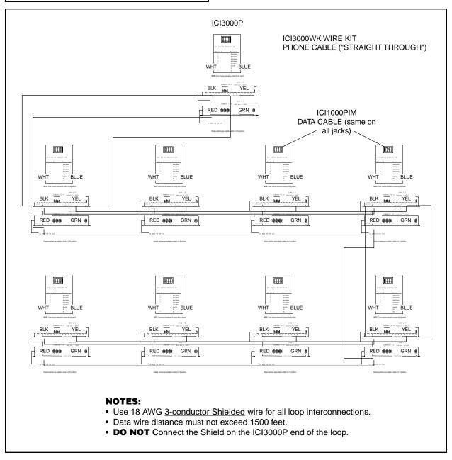
Figure 2. ICI3000P Partyline Wiring Configuration
